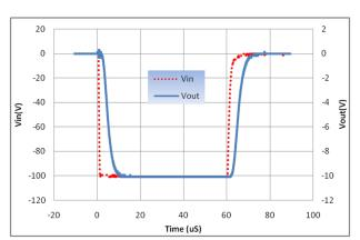
Figure 13: 1000V Input Step Response
