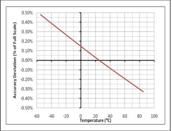
Figure 6: Gain Percentage Deviation vs. Temperature
