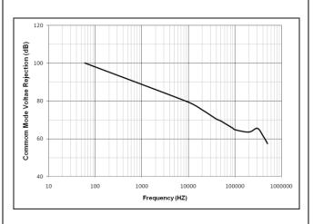
Figure 15: 1000V Common Mode Rejection Response
