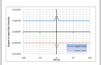
Figure 3: Voltage Sensing Overall Accuracy
