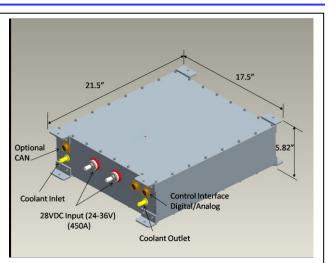
The DC28V850-12KW-UD is an isolated 12KW DC to DC converter that converts nominal 28Vdc (24V to 36V) wide range input DC to 800V Output DC (0 to 850V Adjustable). The high voltage output is protected for over load and short circuit by voltage/current cross regulation. The output current limit can be programmable between 0 to 18A for various applications. Nominal power conversion efficiency is 92%.
